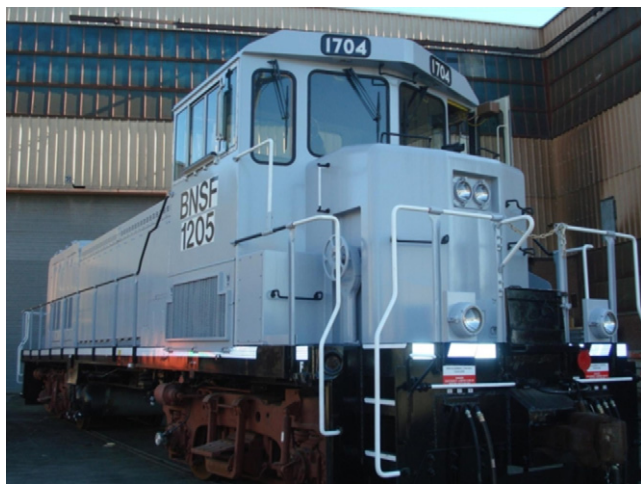
Fig. 1. Fuel cell-hybrid switcher platform vehicle. As shown, the diesel fuel tank and genset have been removed in preparation for retrofitting the fuel cell power plant and hydrogen storage. (Photo courtesy of RailPower Hybrid Technologies.)
